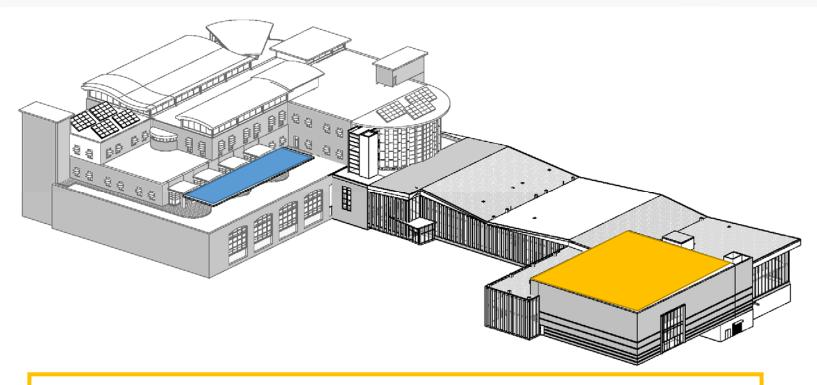
How many standard size panels can fit on top of the MP room? **320 standard panels** (104 kW)
